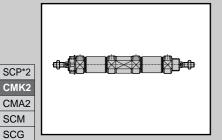
Medium bore size cylinder Double acting back to back type
