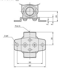
\* Use the body set screws if fixing without a mounting plate. (Thread size: M4 depth 8 pitch 19)
