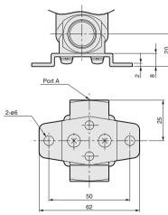
\* Use the body set screws if fixing without a mounting plate. (Thread size: M4 depth 8 pitch 19)
