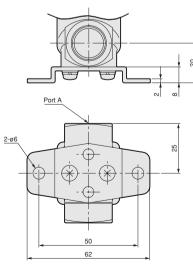
\* Use the body set screws if fixing without a mounting plate. (Thread size: M4 depth 8 pitch 19)
